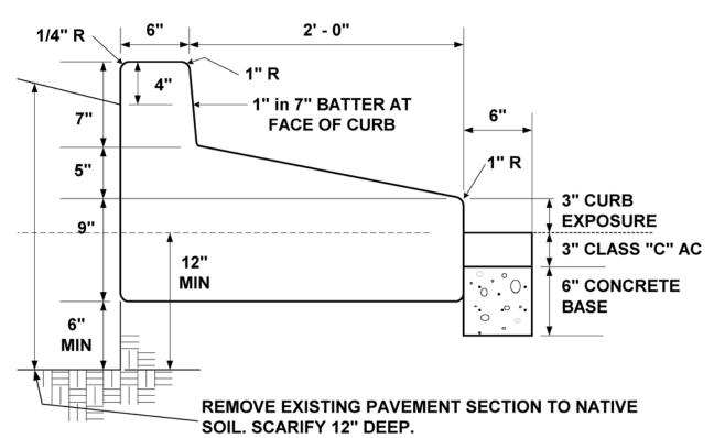
BACKFILL WITH TOPSOIL PLACED IN 9" MAXIMUM LIFTS. COMPACT EACH LIFT WITH 200 POUND GARDEN ROLLER. MOUND TOPSOIL AT CENTER 2" ABOVE TOP OF CURB.
