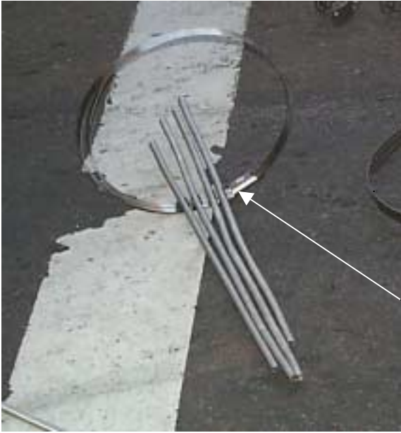
Figure 5. The steel band, mounting clips, and sections of conduit
