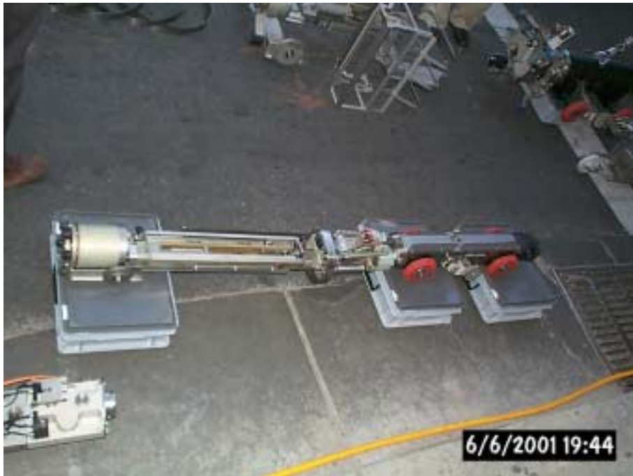
Figure 1. The CityNet robot, ready to inspect sewer lines
