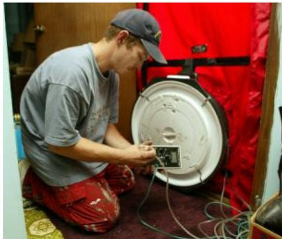
A contractor performing a blower door test to identify air infiltration and leakage throughout a home. [Energy Trust of Oregon](#)
