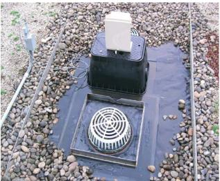
Metro Ecoroof Monitoring Equipment at the Roof Drain
