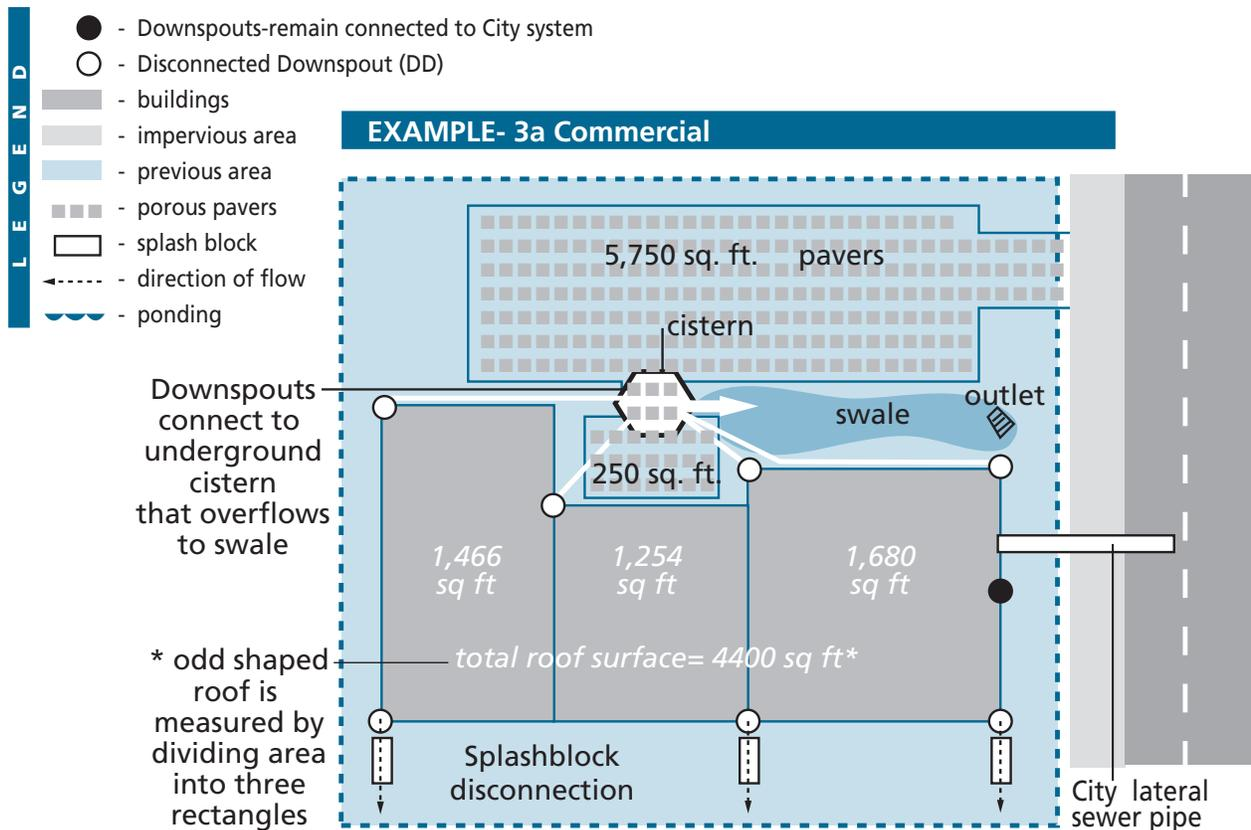
from within the cost range per square foot of facility on the chart on page 8. For this example, the swale range is \$0.45 to \$22.50. We will use a higher value of \$20 per square foot because of demolition required to install the swales. The pavers, cistern and splashblock disconnections bring the total cost to about \$43,570.
