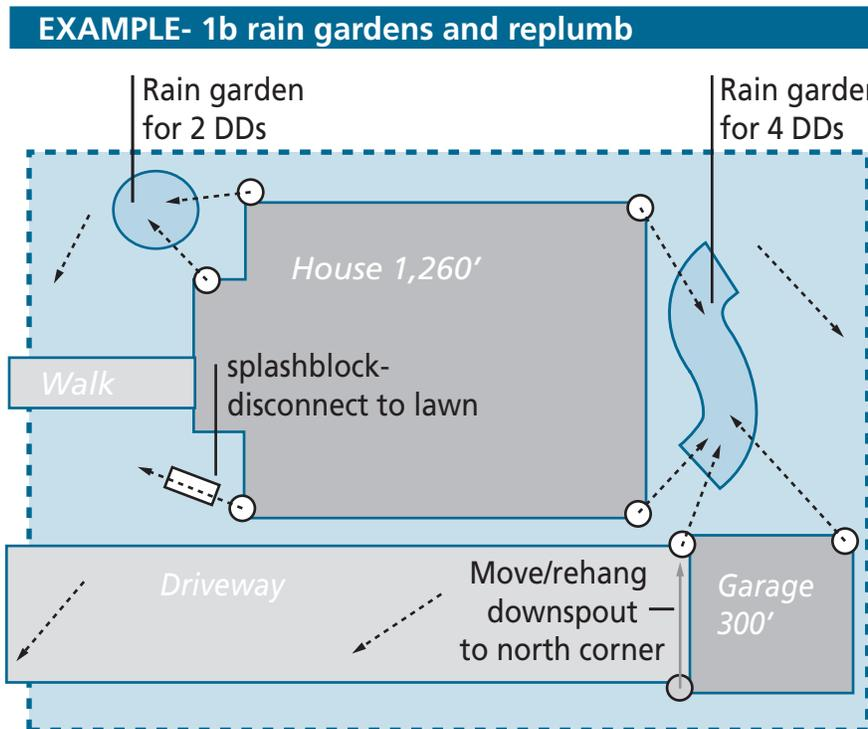
Example 1b will cost a little more. Rehangging the gutter will cost about \$100, and upsizing the rain garden (\$10.50 times the additional 14 square feet) will cost \$147, for a total new cost of \$1,560.50.
