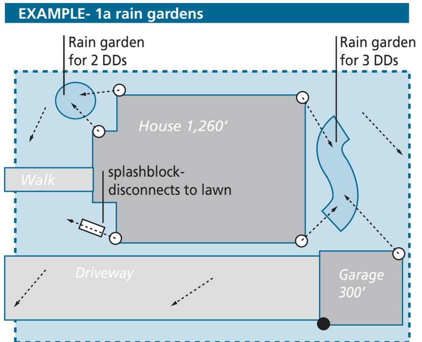
The back rain garden takes drainage from the full back half of the roof and also half of the garage roof. That's 600 square feet of house roof plus 150 square feet of garage roof for a total of 750 square feet. The rain garden needs to be 9% of that area or 67.5 square feet. Round it up to 68, and a 4 foot by 17 foot rectangular space will work.
