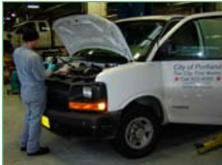
CityFleet uses extended-life antifreeze in its vehicles, which lasts about three times as long as conventional antifreeze.
